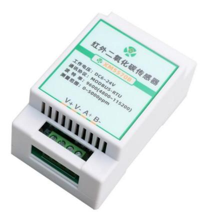
XM5570 using the standard RS485 bus MODBUS-RTU protocol, easy access to PLC, DCS and other instruments or systems for monitoring carbon dioxide state quantities. The internal use of high-precision sensing core and related devices to ensure high reliability and excellent long-term stability, can be customized RS232,RS485,CAN,4-20mA,DC0~5V\10V,ZIGBEE,Lora,WIFI,GPRS and other output methods.
