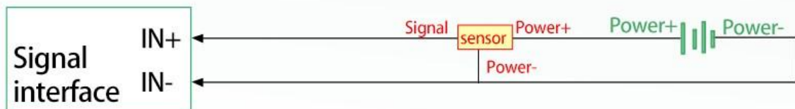
Differential wiring diagram of the current three-wire system
