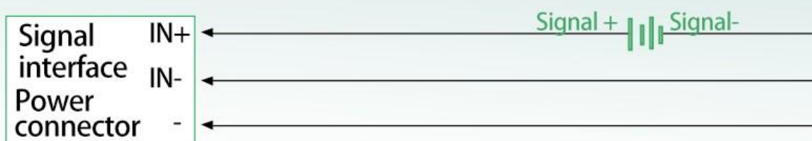
Single-ended wiring diagram for voltage acquisition
