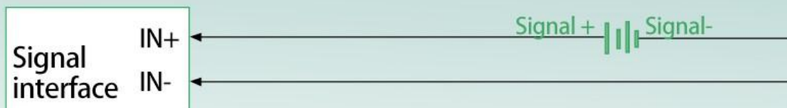
Voltage acquisition differential wiring diagram
