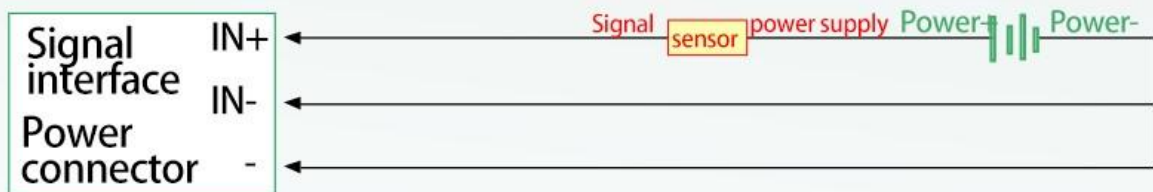
Single-ended wiring diagram of the two-wire current system
