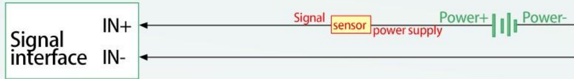
Differential wiring diagram of the two-wire system of current
