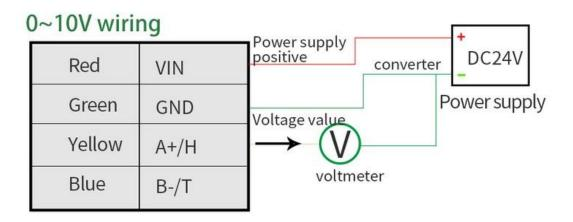
In the case of broken wires, wire the wires as shown in the figure. If the product itself has no leads, the core color is for reference.
