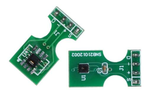
YH0230 using the standard ,easy access to PLC, DCS and other instruments or systems for monitoring \_11\_15\_20\_21\_25\_30\_31\_35 state quantities. The internal use of high -precision sensing core and related devices to ensure high reliability and excellent long-term stability,can be customized RS232,RS485,CAN,4-20mA,DC0~5V\10V,ZIGBEE,Lora,WIFI,GPRS and other output methods.
