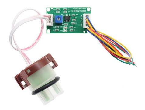
other instruments or systems for monitoring 浊度 state quantities. The internal use of high-precision sensing core and related devices to ensure high reliability and excellent long-term stability, can be customized RS232,RS485,CAN,4-20mA,DC0~5V\10V,ZIGBEE,Lora,WIFI,GPRS and other output methods.
