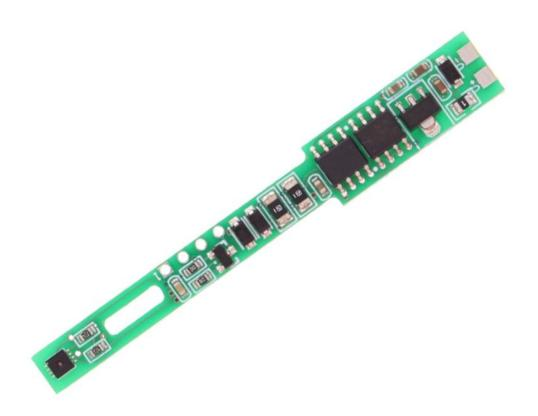
YM7820B using the standard RS485 bus MODBUS-RTU protocol, easy access to PLC, DCS and other instruments or systems for monitoring temperature, humidity state quantities. The internal use of high-precision sensing core and related devices to ensure high reliability and excellent long-term stability, can be customized RS232,RS485,CAN,4-20mA,DC0~5V\10V,ZIGBEE,Lora,WIFI,GPRS and other output methods.
