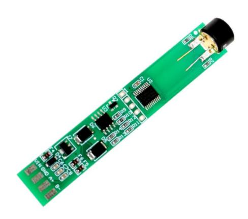
YM8701 using the standard ,easy access to PLC. DCS and other instruments or systems for monitoring temperature state quantities. The internal use of high-precision sensing core and related devices to ensure high reliability and excellent long-term stability, can be customized RS232,RS485,CAN,4-20mA,DC0~5V\10V,ZIGBEE,Lora,WIFI,GPRS and other output methods.
