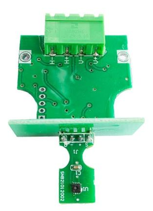
YN1810C using the standard CAN Bus,easy access to PLC, DCS and other instruments or systems for monitoring temperature,humidity state quantities. The internal use of high-precision sensing core and related devices to ensure high reliability and excellent long-term stability,can be customized RS232,RS485,CAN,4-20mA,DC0~5V\10V,ZIGBEE,Lora,WIFI,GPRS and other output methods.
