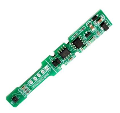
YN7320B using the standard RS485 bus MODBUS-RTU protocol, easy access to PLC, DCS and other instruments or systems for monitoring temperature, humidity state quantities. The internal use of high-precision sensing core and related devices to ensure high reliability and excellent long-term stability, can be customized RS232, RS485, CAN, 4-20mA, DC0~5V\10V, ZIGBEE, Lora, WIFI, GPRS and other output methods.
