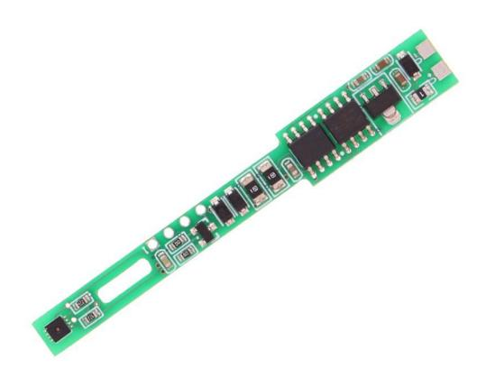
YN7820 using the standard RS485 bus MODBUS-RTU protocol, easy access to PLC, DCS and other instruments or systems for monitoring temperature, humidity state quantities. The internal use of high-precision sensing core and related devices to ensure high reliability and excellent long-term stability, can be customized RS232,RS485,CAN,4-20mA,DC0~5V\10V,ZIGBEE,Lora,WIFI,GPRS and other output methods.
