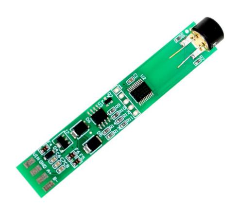
YN8701 using the standard ,easy access to PLC, DCS and other instruments or systems for monitoring temperature state quantities. The internal use of high-precision sensing core and related devices to ensure high reliability and excellent long-term stability, can be customized RS232,RS485,CAN,4-20mA,DC0~5V\10V,ZIGBEE,Lora,WIFI,GPRS and other output methods.
